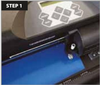
Feed your material into the cutter with the mylar carrier facing down.
