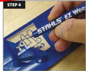
Weed always excess material, leaving only the design on the mylar carrier.
